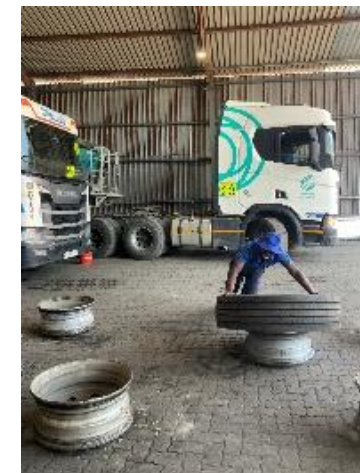
Photo 8 Employee throwing truck tyre forcefully over rim in order to go over the sides of the rims
