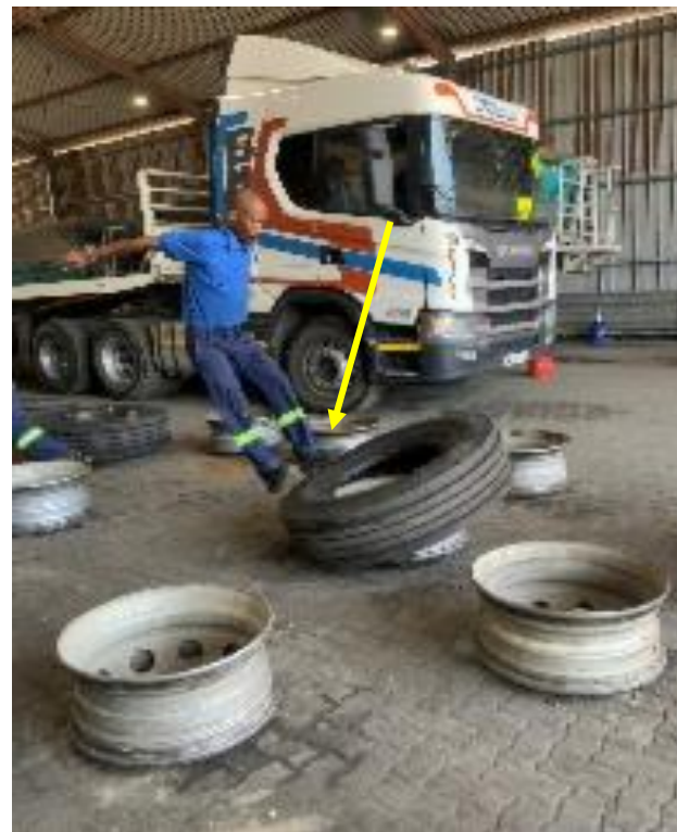
Photo 9 Employee jumping onto tyre trying to put the tyre on the rim
